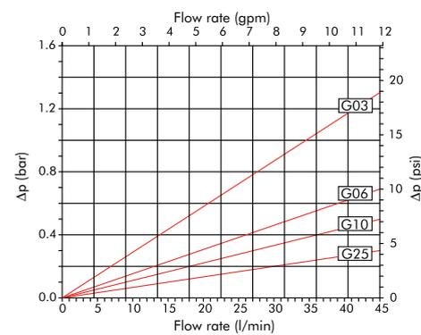
The above diagrams have been obtained at the FILTREC laboratory, according to the ISO 3968 specification, with mineral oil having 30 cSt viscosity and 0,86 Kg/dm<sup>3</sup> density.
